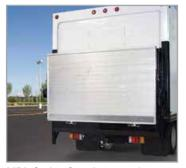
MDL Series Gate in stowed position
