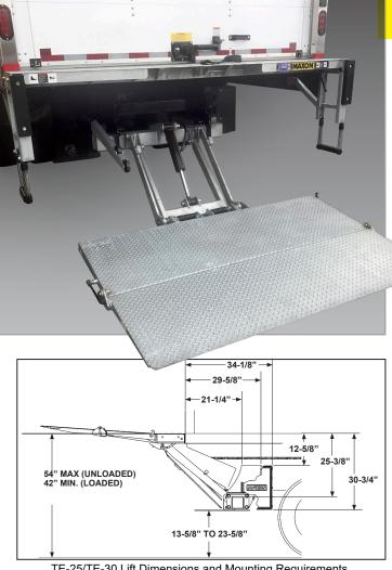
TE-25/TE-30 Lift Dimensions and Mounting Requirements
