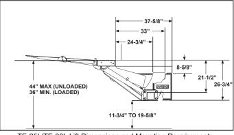
TE-25L/TE-30L Lift Dimensions and Mounting Requirements
