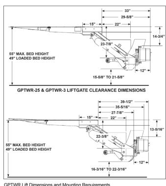
**GPTWR Lift Dimensions and Mounting Requirements**
