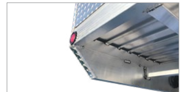
Rear Light - Underside (No Exposed Wiring)
