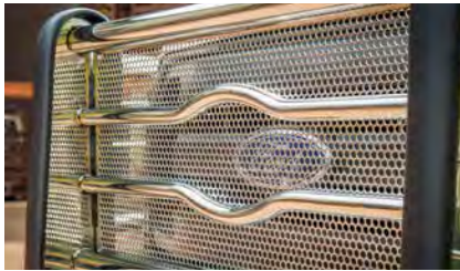
Heavy-gauge, punched steel screen provides extra grille protection
