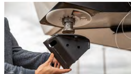
Head piece bolts onto kingpin, allowing head channel to guide the kingpin into place for easier hookup
