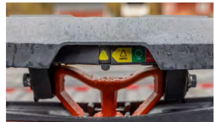
Three-position coupling indicator clearly shows coupling status
