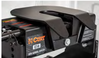
Features an anti-rattle skid plate to help reduce noise
