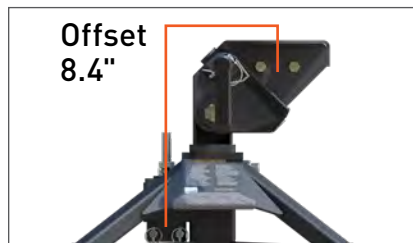
Coupling point offsets 8.4" rearward for added turning clearance (16051 / 16602 only)
