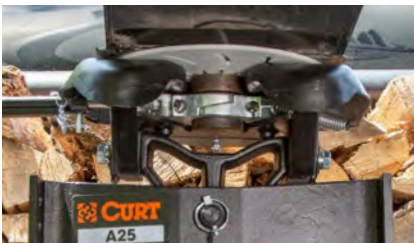
Adds a buffer between 5th wheel head plate and kingpin box
