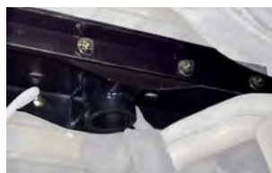
Step 2 - Fully install brackets and hitch to the vehicle frame
