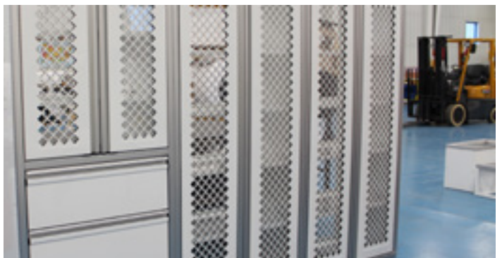
Locker Door Venting
