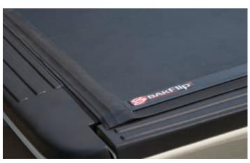
EPDM RUBBER SIDE SEALS KEEPTHE ELEMENTS OUT
