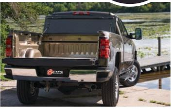
PROP RODS SECURE COVER IN FLIPPED UP POSITION
